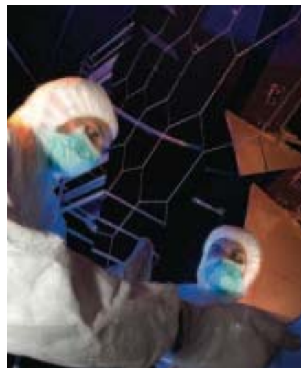
Assembly of a ring-imaging Cherenkov detector for the LHCb detector is carried out under extremely clean conditions.
