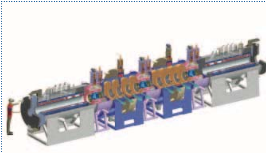
An engineering drawing of the Muon Ionisation Cooling Experiment (MICE) at the CCLRC Rutherford Appleton Laboratory in the UK. This experiment is an essential step in R&D towards the realization of a neutrino “factory”.
