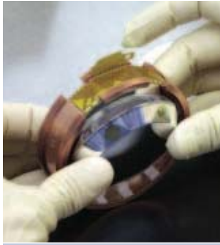
The Edelweiss experiment in the underground laboratory at Modane in France searches for particles known as WIMPs with detectors made from germanium.
